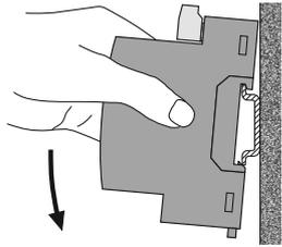
Fig. 1. Mounting on top-hat rail 35 x 15 or 35 x 7.5 mm.
