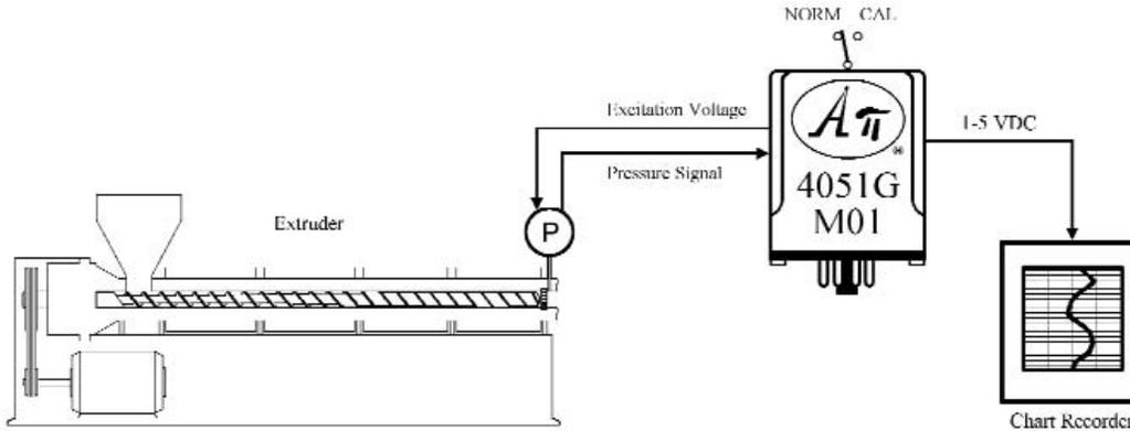
The API 4051 G M01 has an internal calibration resistor to unbalance a 350 ohm bridge to an 80% of span value when the test switch is in the CAL position, allowing for convenient and accurate calibration.
