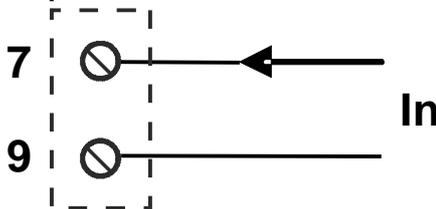
When connected to a current transformer, one of the two wires must be grounded.
