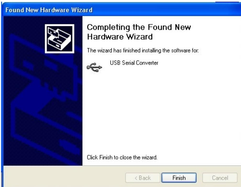
Once pressed the "Finish" button, the driver for the S117P1 converter has been installed. Now the second part of the installation begins: from now on, the **virtual driver** will be installed, and all the programs will use the converter as a standard serial port. The following signalling will appear, and a similar to the former procedure will begin:
