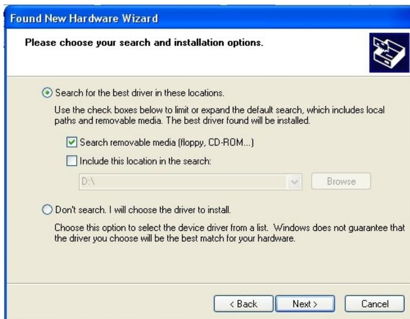
Select the first option, and the operating system will find the best driver for the device in the path chosen. In case the CD is not present in the CD-Rom device, please insert the mini-CD provided in the box, select the “**Search removable media**” and click “**Next**”. Once the correct driver has been found, the following window will appear:
